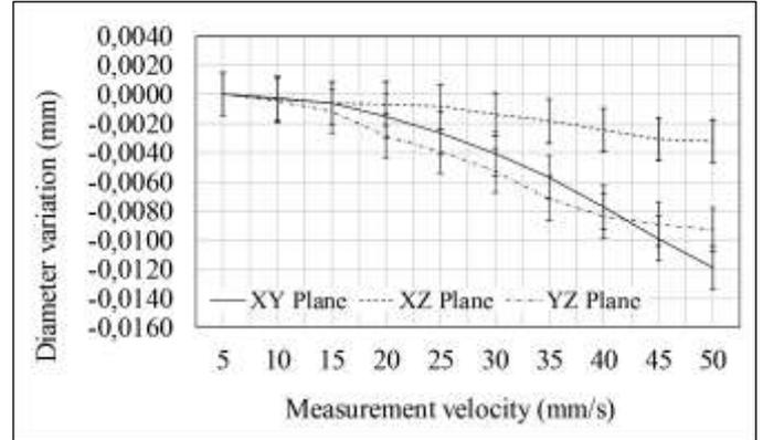
Fig. 7. Influence of velocity on measured diameter – 3-axis mode.
