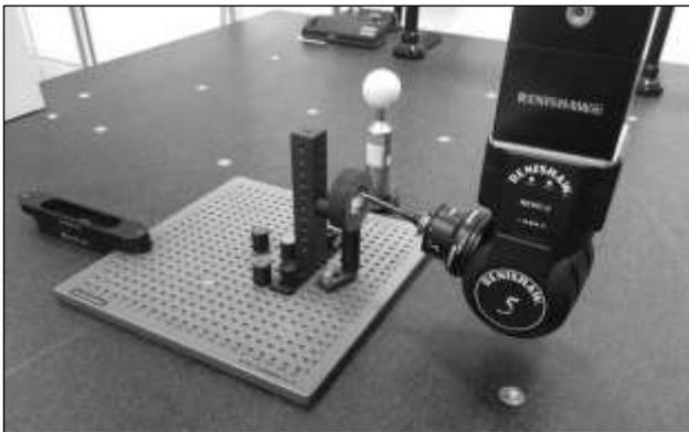
Fig. 9. CMM with rotary scanning probe.
