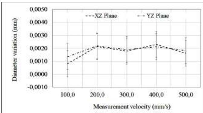
Fig. 12. Diameter measured at very high speed scanning – 5-axis mode.
