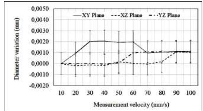
Fig. 10. Influence of velocity on measured diameter.
