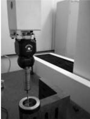
Fig. 6. CMM with fixed scanning probe.
